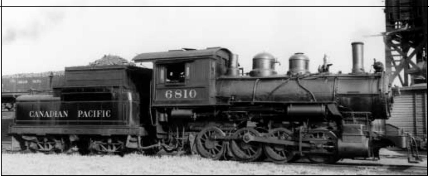
The 6810 was photographed in Vancouver on April 28, 1939 and demonstrates why this class is so interesting to study. This locomotive has the original Baldwin domes and yet another style of whistle and pop valve dome. The tongue-and-groove window filler on the cab shows clearly in this photograph. The engine has a 3,400 gallon tender from a 70" driver Ten-Wheeler such as an E4.
