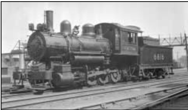
This fireman side view of 6816 appears to be taken during the early part of the Second World War, most likely in Vancouver because the headlight has been removed and the smaller black-out style fitted. This another example of the diversity of the hardware used on the Via switchers. This locomotive has a combination of a Baldwin steam dome and a normal CP sand dome. Just to be unique, this engine does not have the usual CP bell-boiler feed water valve assembly. Instead, this engine has a simple bell mount between the domes and the boiler feed water at the side just above the air tank, an arrangement that would be similar to when the engine was built. The engine appears to have a 4,000 gallon tender.
